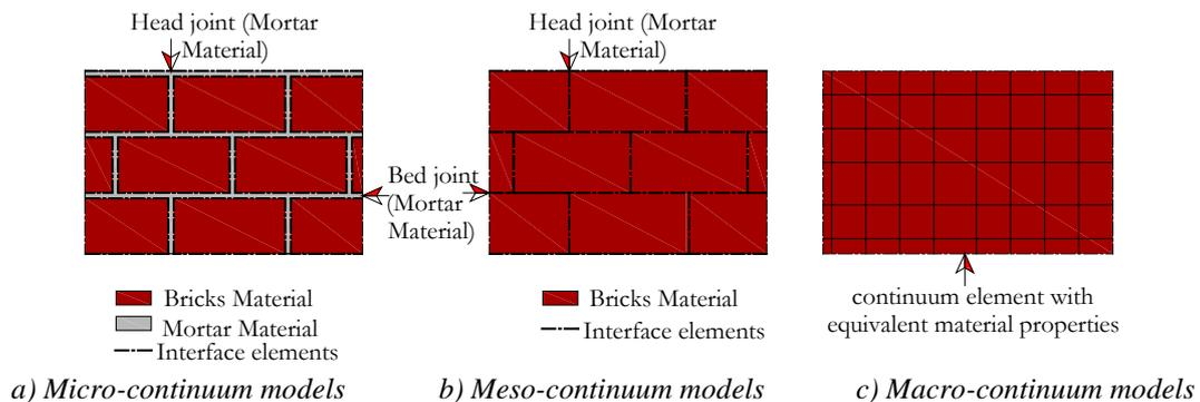
Figure 3 Continuum modelling approaches for masonry infills
