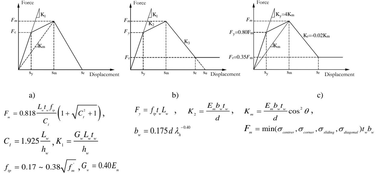
where  $f_m'$  is the masonry compressive strength in MPa,  $d$  is the diagonal length of the infill and  $b_w$  is the width of the strut,  $\sigma_{center}$  crushing stress at the centre of the panel,  $\sigma_{corner}$  crushing stress of the panel corner,  $\sigma_{sliding}$  sliding stress at the horizontal mortar joints and diagonal tensile stress  $\sigma_{diagonal}$
