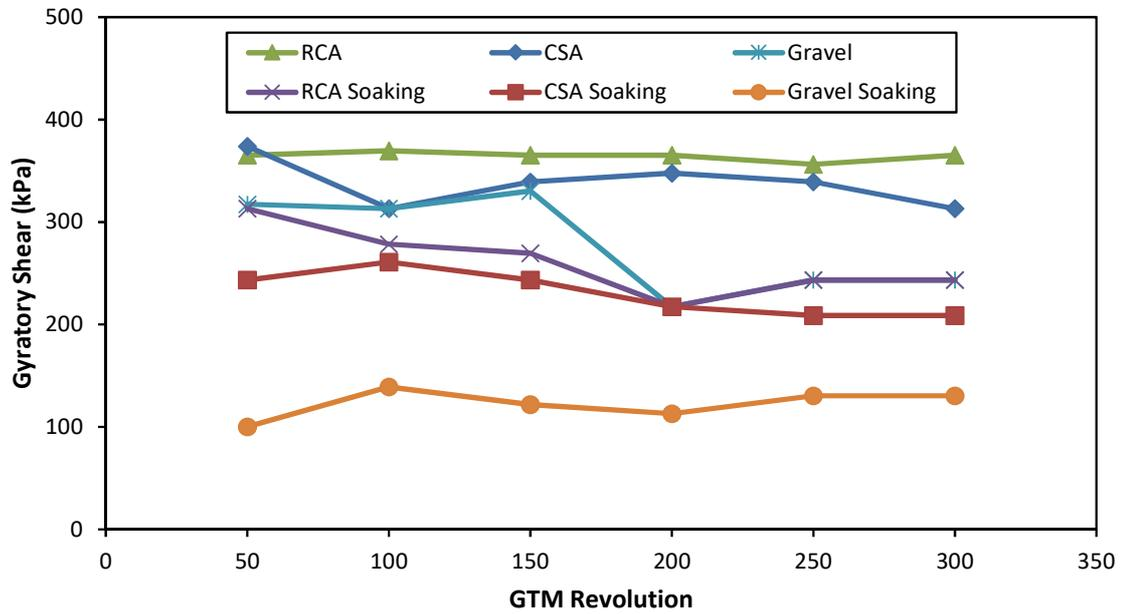
Figure 3 - Evolution of gyrotory shear with GMT revolutions for different aggregates (adapted from Park, 2003).
