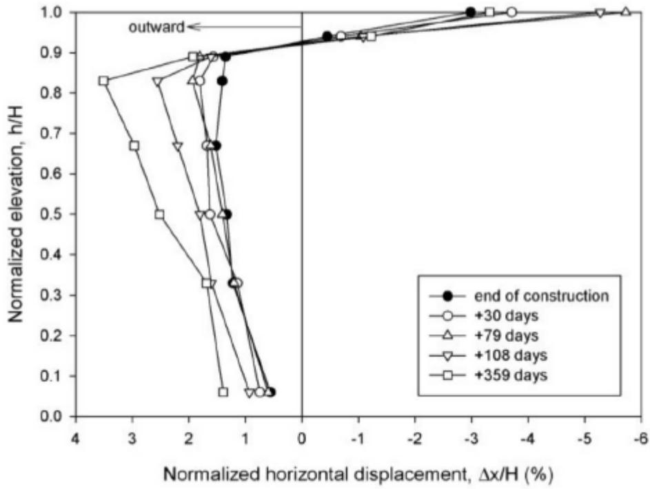
Figure 5 – Normalized horizontal displacements of the wall face recorded by Santos et al. (2013).
