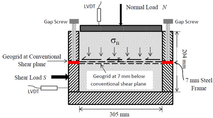
Figure 6 – Modified lower direct shear box with steel frame (Arulrajah et al., 2013b).
