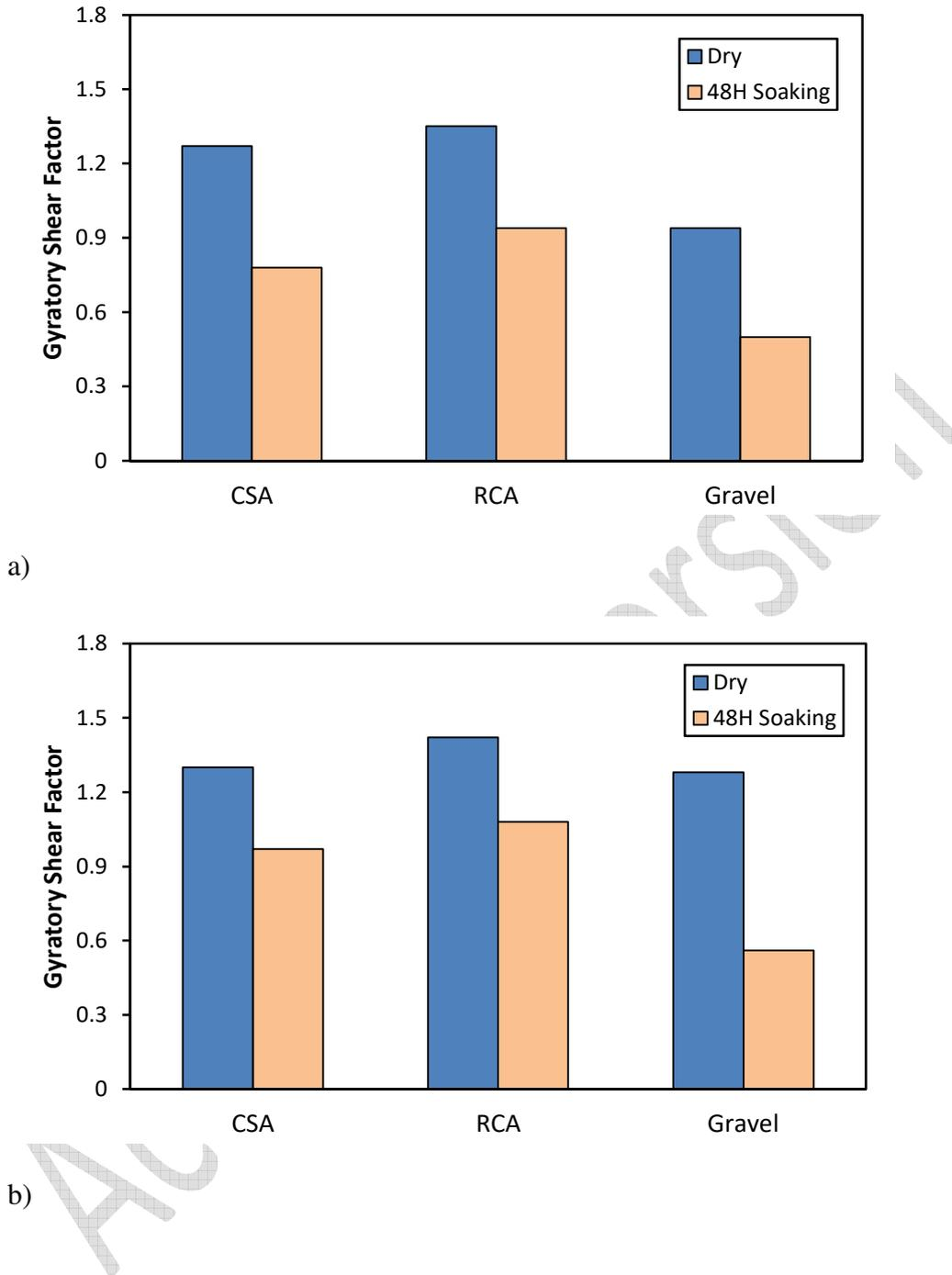
Figure 2 - Comparison of gyratory shear factor for different aggregates (Park, 2003):
