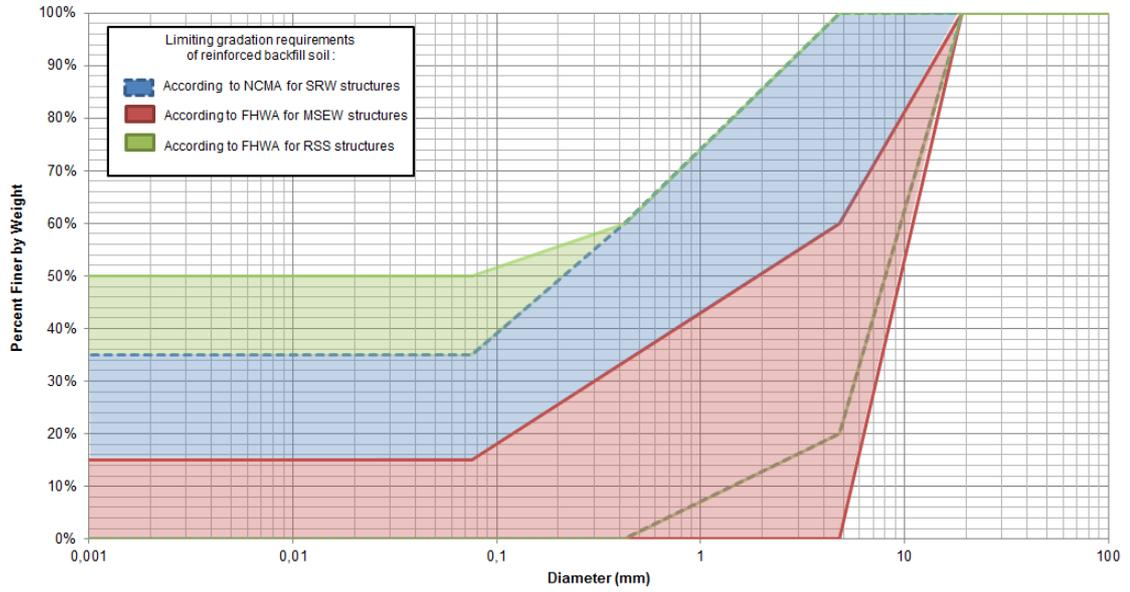
Figure 1 - Particle sizes recommended by FHWA (2010) and NCMA (2010).
