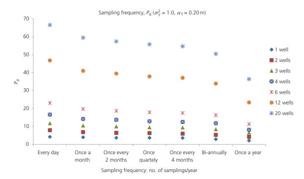
Figure 6. Probability of detection,  $P_d$ , plotted against the frequency of sampling for a mild heterogeneous medium (variance of In K is equal to 1, where K is the hydraulic conductivity and transverse dispersivity,  $\alpha_T$ , is equal to 0.2 m) for several configurations of monitoring wells (Papapetridis and Paleologos, 2011b)
