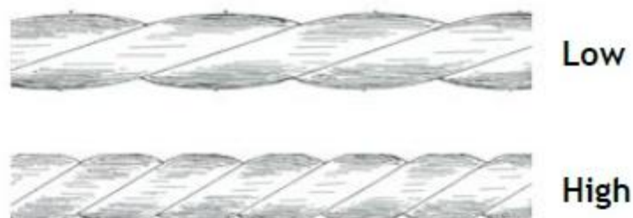
Figure 3 - Appearance of a cord with low and high twist level (adapted from [7]).
