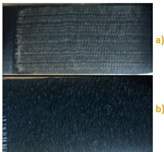
Figure 6 - Coverage in peel adhesion samples: a) no coverage, b) full coverage.
