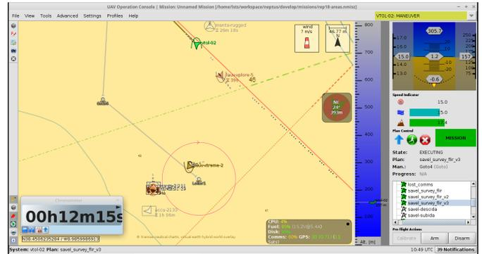
Fig. 7: Neptune console screenshot in AUV and UAV coordinated operation.
