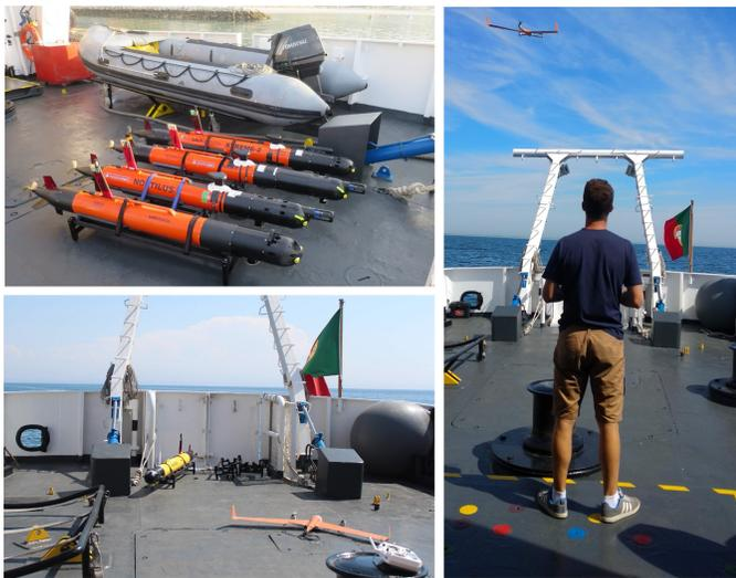
Fig. 1: Some of the hardware used by LSTS. Bottom mapping AUVs (top-left), Water column AUV next to VTOL UAV (bottom-left) and VTOL UAV being launched from NRP Auriga (right).
