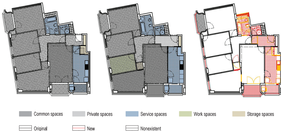
Figure 7. (apartment 3, typology B, 4 th floor). Floor plans: original, current and alterations. Scale 1:250
