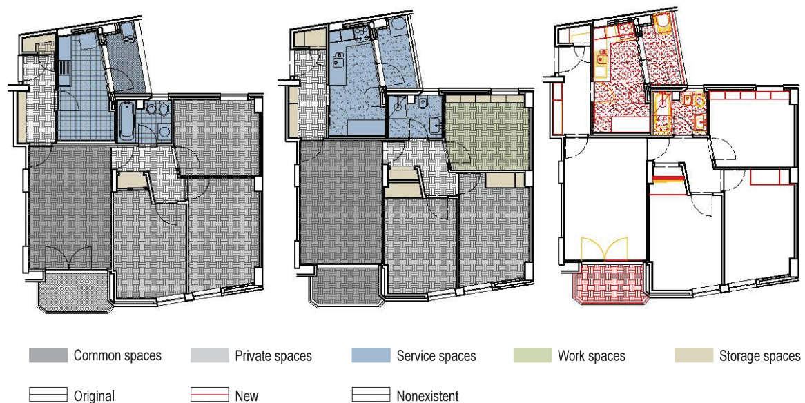
Figure 3. (apartment 1, typology A, 6 th floor). Floor plans: original, current and alterations. Scale 1:200
