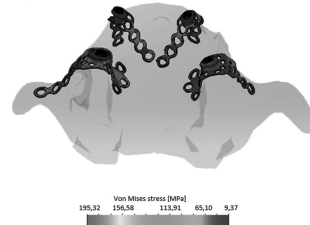
Figure 4. Stress distribution on plates [MPa].
