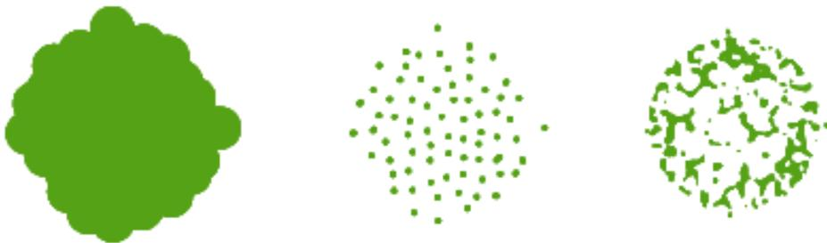
Figure 4.4: Different cross sections of a model for 3D printing as seen in the printable file. Cross section relative to the bottom layers (left), cross section relative to the initial generated supports (center), cross section relative of one model layer (right).
