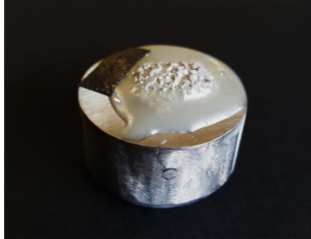
Figure 3.3: 3D porous sample prepared for scanning electron microscopy.
