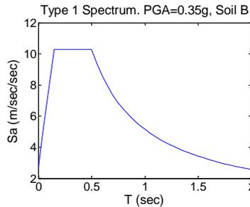
Fig. 2 – Elastic response spectrum used for the analyses.
