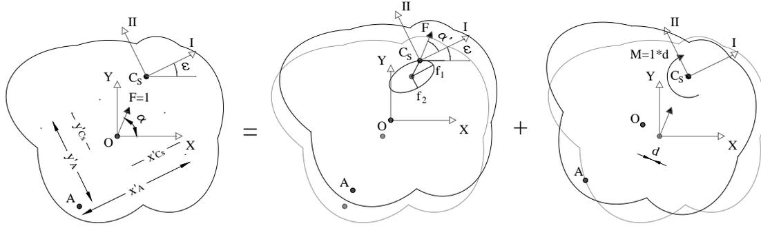
Fig. 1 – Displacement of a single storey building subjected to a horizontal unit static force applied at  $O$  with an arbitrary direction  $\alpha$  with respect to the structural axis  $X$ .
