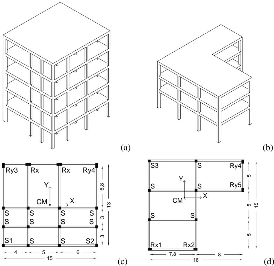
Fig. 3 – 3D representation of the 5-storey structure (a) and the 3-storey structure (b) and their typical plan views (c), (d), respectively (dimensions in m).
