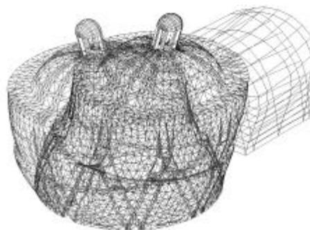
**Figure 10: Peak displacement envelopes from linear elastic analysis**
