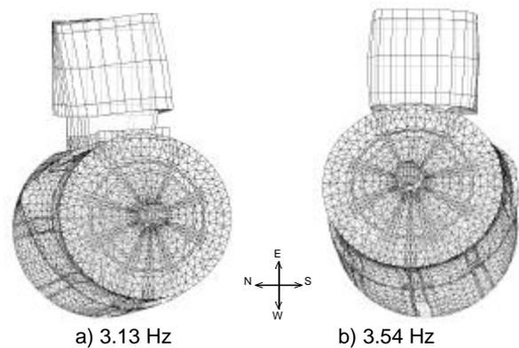
**Figure 9: 1<sup>st</sup> and 2<sup>nd</sup> vibration modes, numerically obtained (plan view)**
