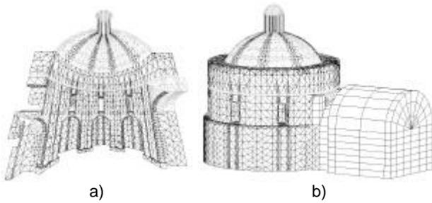
**Figure 3: Numerical modeling of the church. (a) Half-mesh (inside view) and (b) total mesh (outside view)**
