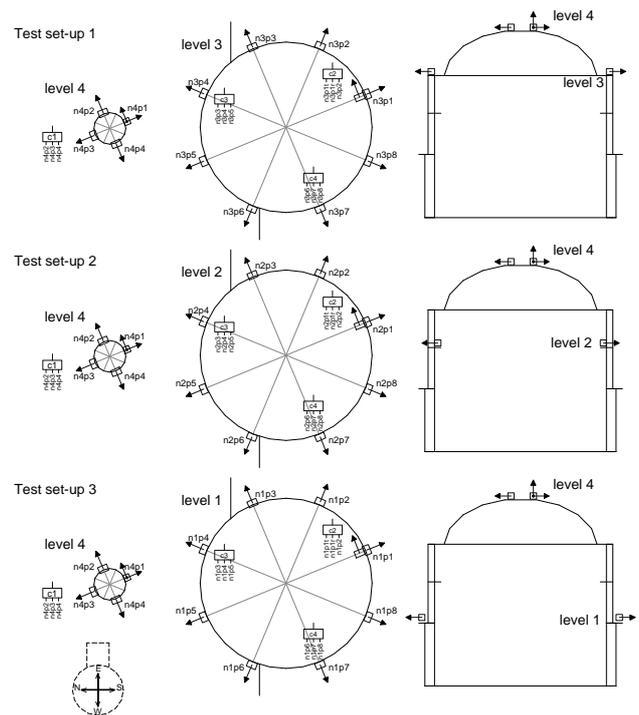
**Figure 4: Instrumented points for the three different testing configurations**
