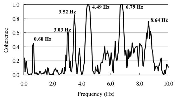
**Figure 7: Coherence between records at points n4p3 (level 4) and n1p5 (level 1)**
