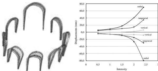
**Figure 12: a) Maximum deformed shape of arches and columns; b) Vulnerability functions of arch displacements**
