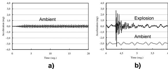
**Figure 5: Response of the n1p2 accelerometer due to (a) ambient vibration and (b) explosion**
