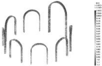
**Figure 11: Maximum tensile stresses (1.15 MPa) in blocks of arches and columns (intensity 2.4)**
