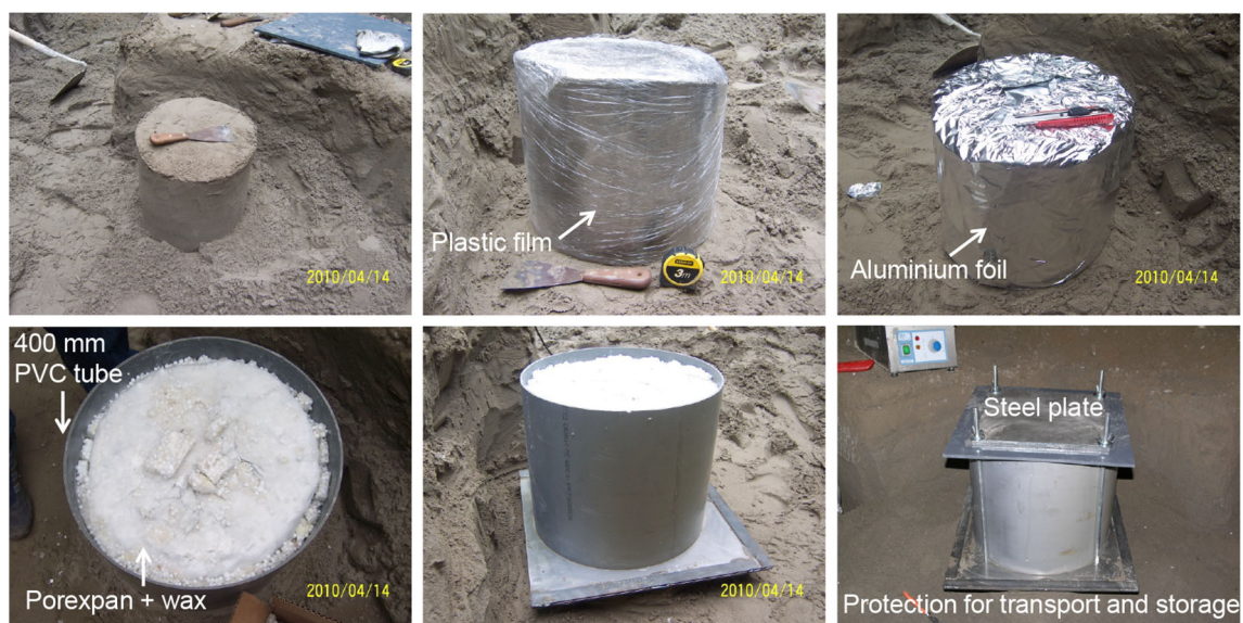
Fig. 24 Block sampling in silty deposits from the Llobregat River, Barcelona (Spain)
