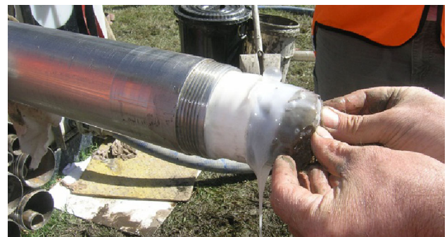
Fig. 9 Lubricating polymer gel coating soil sample (from [66])
