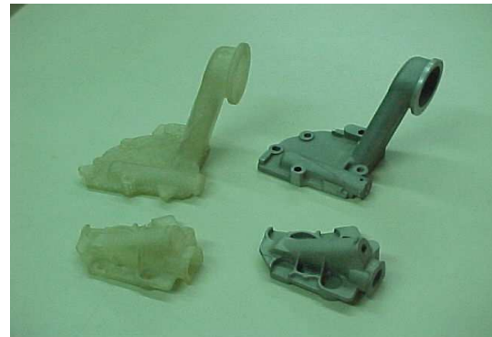
Fig. 2. SLA models and prototypes in an aluminium alloy, obtained by the lost Quick Cast process.
