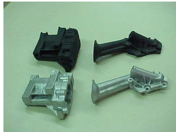
Fig. 3. Wax model (Thermoject) and aluminium prototypes obtained by the lost wax process.
