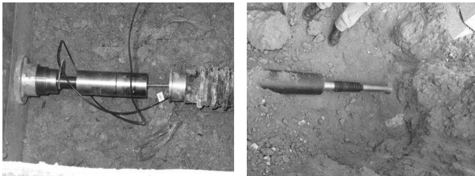
Figure 13. Installation of the Long Gauge sensors: (a) detail of the tension mechanism; (b) anchoring and protection.
