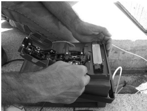
Figure 18. Coupling: (a) fusion splice; (b) butt-joint connection.
