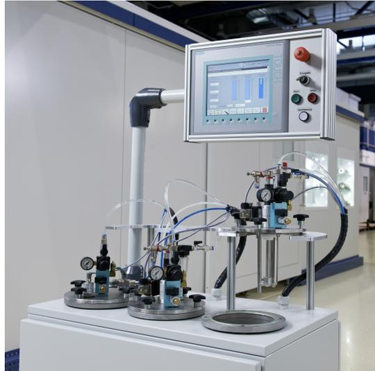
Figure 2.10: Three-vessels suspension feeder (Fraunhofer IWS) [119]
