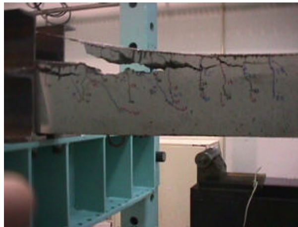
Fig. 9. Rupture of the reinforced beam
