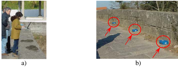
Figure 3: Dynamic test. a) System configuration phase. b) Positions of three macro-seismographs on the bridge.
