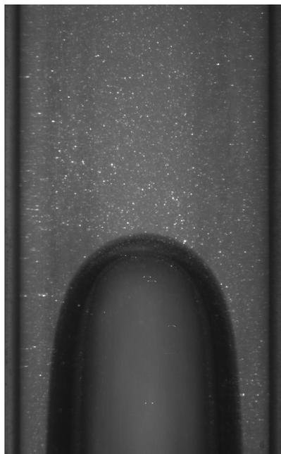
Figure 6. Simultaneous PIV and shadowgraphy image of a Taylor bubble (gas slug)
