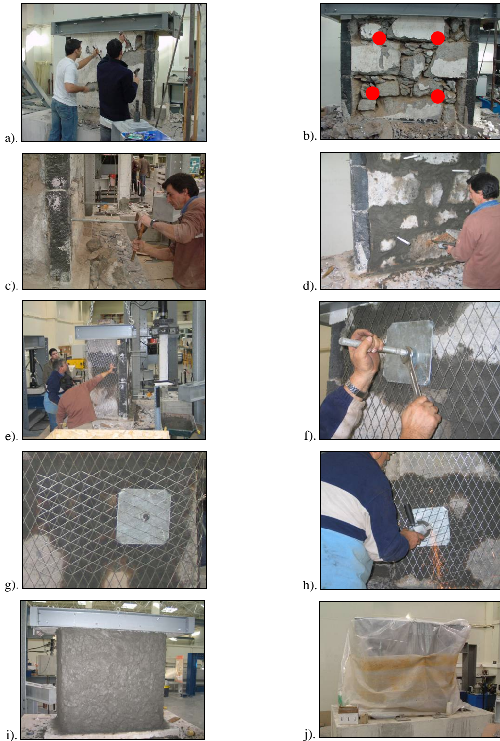
Figure 11: Retrofitting technique: a) cover removal; b) position of the steel rods; c) placement of the rods; d) mortar (1 st phase); e) installation of the steel mesh; f) placement of the steel plates and tightening; g) installation of the steel mesh above the plates; h) cutting the excess of steel rods; i) mortar cover (2 nd phase); j) mortar cure simulating Azores' humidity
