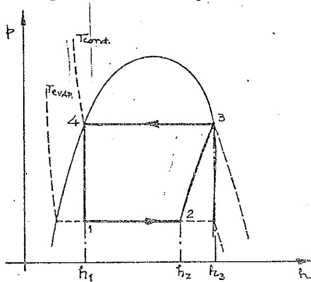
$$h_4 = h^*(30^\circ\text{C}) = 447.862 \text{ kJ/Kg} = h_1$$
