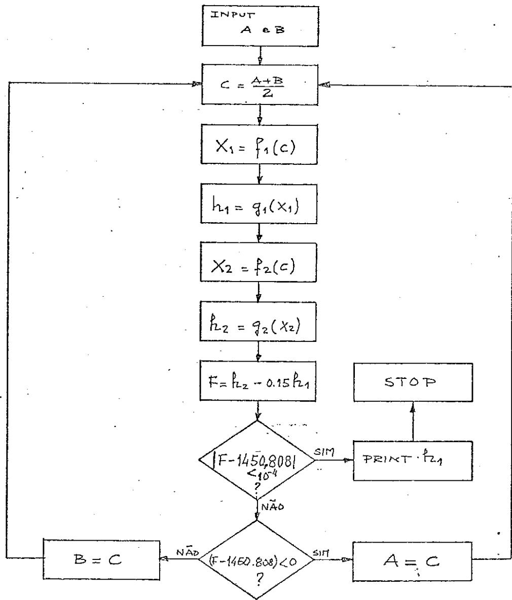
$$X_1 = \frac{C - 3.473}{5.9515} \quad h_1 = 237.810 \cdot (1 - X_1) + 1524.897 \cdot X_1 \quad [\text{kJ/kg}]$$
