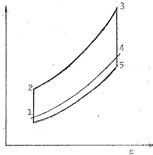
$$W_{\text{comp}} = -C_p (T_2 - T_1)$$
