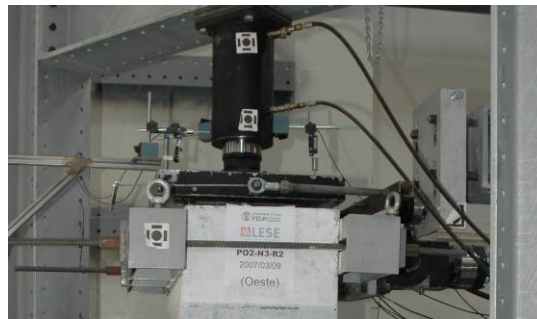
Figure 2: The sliding device used to apply the axial load.
