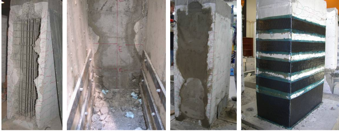
Figure 8: Hollow piers before and after the shear retrofitting with inside steel bars and outside CFRP sheet.
