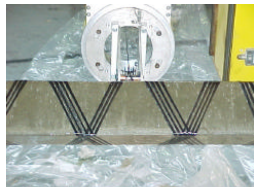
Figure 10. Winding of first layer
