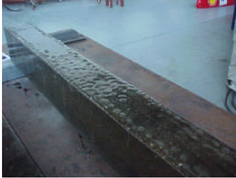
Figure 7. Surface epoxy resin application
