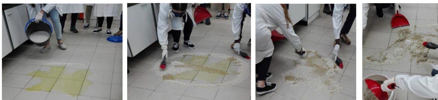
Figure 1. Sequence of images showing the delimitation, covering and collection of the spilled liquid.
