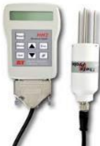
Figure 4.6 The ThetaProbe model ML3 for the measurement of the soil volumetric water content.
