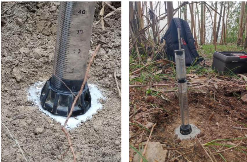
Figure 4.5 Unsaturated hydraulic conductivity measurement in the field with the mini disk infiltrator (MDI).
