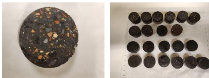
Figure 3.2 Coal mining waste sample, polished blocks for petrological analyses.
