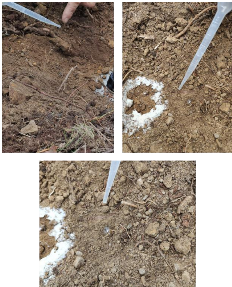
Figure 4.8 Water Drop Penetration Time test (WDPT) in the field.
