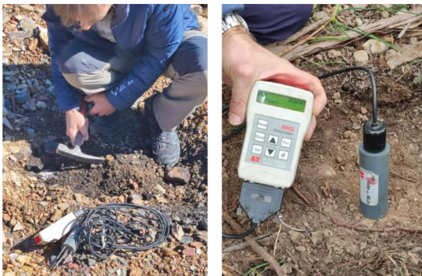
Figure 4.7 Measuring the volumetric soil water content in the study area using the ML3 ThetaProbe.
