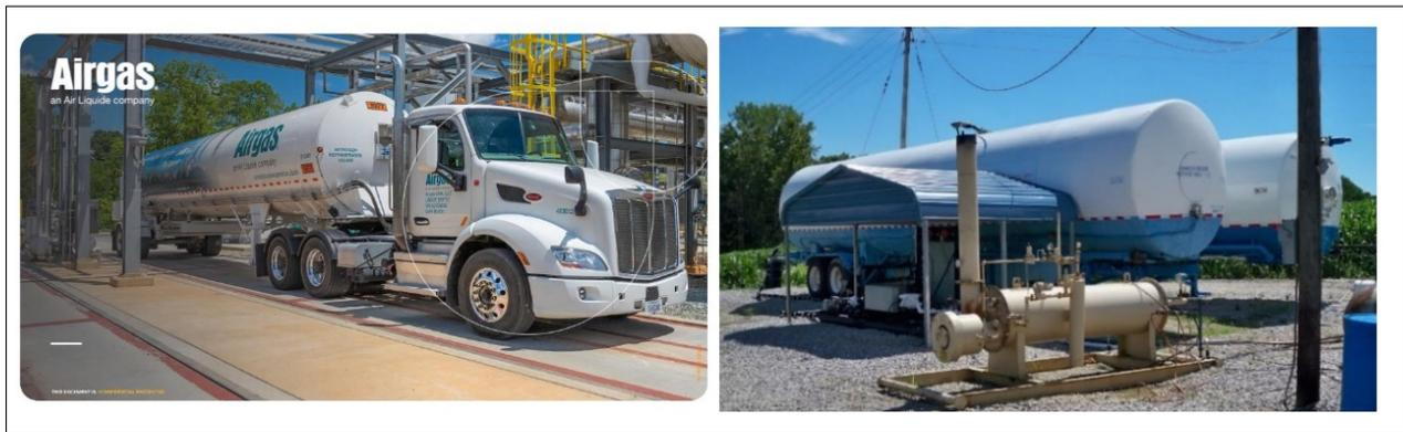
**Figure 19:** Transport truck for refrigerated liquid (left-side) and portable liquid CO<sub>2</sub> storage container (right-side), [12].
