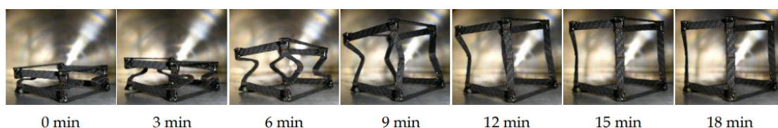
Figure 2.20: Shape recovery sequence of the deployable cube structure [35].
