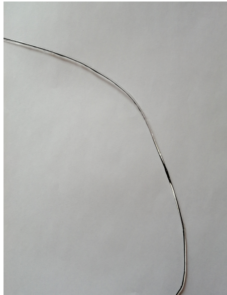
Figure 3.15: CF/PLA filament produced with the first extrusion setup, using a 4mm die
