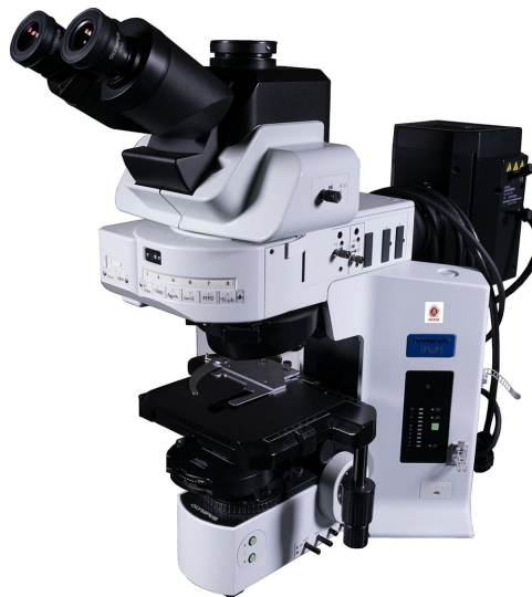
Figure 3.22: Olympus BX61 Motorized Brightfield Darkfield Microscope w/ Laser Autofocus Pred BX63 [45].
