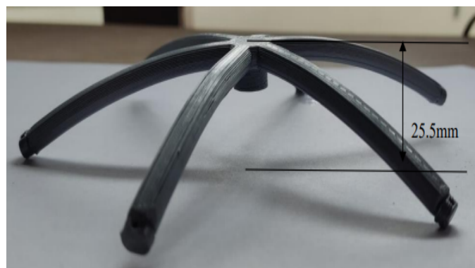
(a) prototype's natural warp, after contact with hot water
