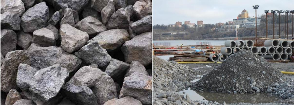
Figure 2.16 - Samples of the *Sprängsten* material used as backfill
