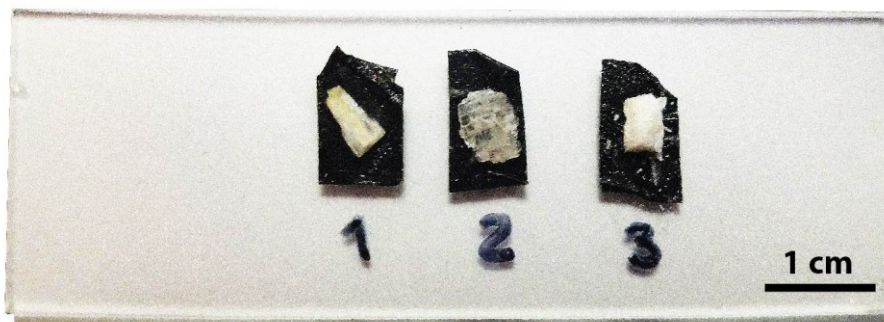
Figure 60. Individual petalite grains mounted on a thin section for cold-cathodoluminescence (CL) observation. 1) petalite from Queiriga, 2) petalite from Gondães and 3) petalite from Gonçalo.
