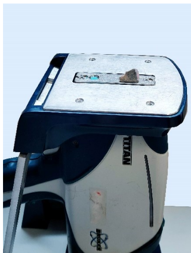
Figure 8. Portable X-Ray Fluorescence (pXRF) device (Bruker S1 Titan 600) used in this study for geochemical analysis of K-feldspar samples, demonstrating its effectiveness for rapidly identifying Li-rich pegmatites in the field.
