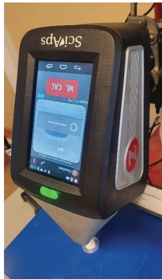
Figure 7. Portable LIBS equipment (Sciaps Z300) used for this study.
