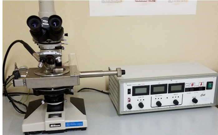
Figure 10. Cathodoluminescence (CL) system: CITL CCL 8200 MK4 with Nikon OPTIPHOT-POL microscope (University of Porto, Faculty of Sciences). Used to verify petalite purity, compare CL features of spodumene and petalite, and explore CL-based image analysis for spodumene quantification.
