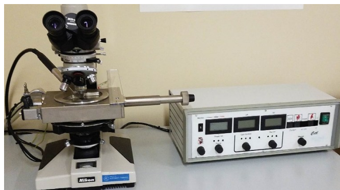
Figure 85. Cold cathodoluminescence microscopy equipment used to verify mineralogical purity of petalite pellets.
