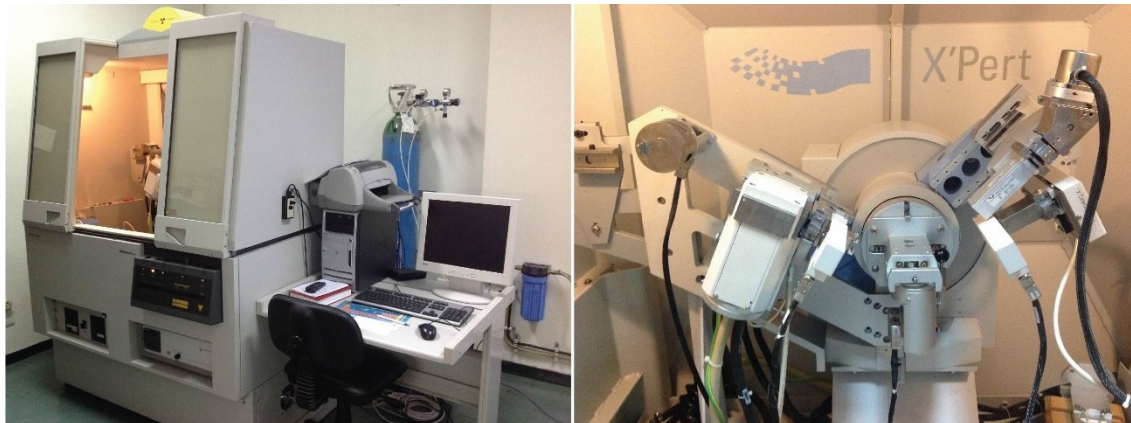
Figure 86. X-Ray Diffraction (XRD) equipment at LNEG (Laboratório Nacional de Energia e Geologia) used for the mineralogical characterization of NIST SRM 182 (petalite).
