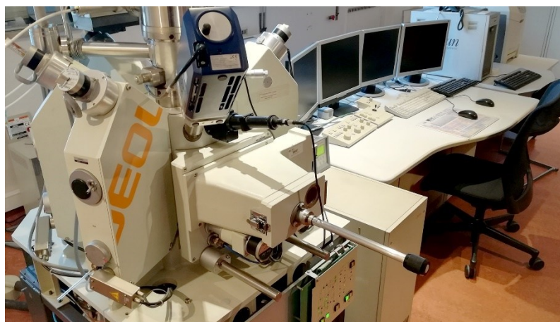
Figure 11. JEOL JXA 8500-F electron microprobe used for EPMA analyses at the National Laboratory of Energy and Geology (LNEG) in S. Mamede de Infesta, Porto, Portugal. This instrument was employed to determine the concentration of silicon (Si) in spodumene and cookeite samples from the Barroso–Alvão field in preparation for LA-ICP-MS analysis.
