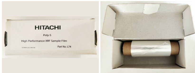
Figure 94. Hitachi Poly-S High Performance XRF Sample Film (3.5 μm) tested for the analysis of K-feldspar crystals.
