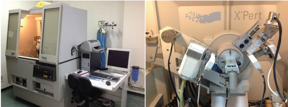
Figure 12. X-ray powder diffraction (XRD) setup used for the mineralogical characterization of SRM 182 at the National Laboratory of Energy and Geology (LNEG), S. Mamede de Infesta, Portugal. The instrument shown is a Panalytical Diffractometer XPERT-PRO, equipped with a PW3050/60 goniometer, with a Theta-2Theta geometry and X-ray tube with a copper (Cu) anticathode.
