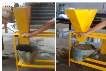
Fig. 5. (a) Filling the funnel; (b) Opening the gate.
