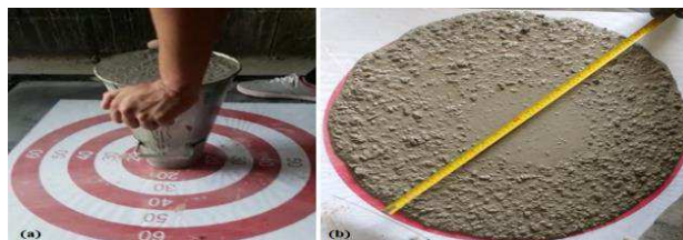
Fig. 1. (a) Abrams cone filled; (b) Scattering measurements.
