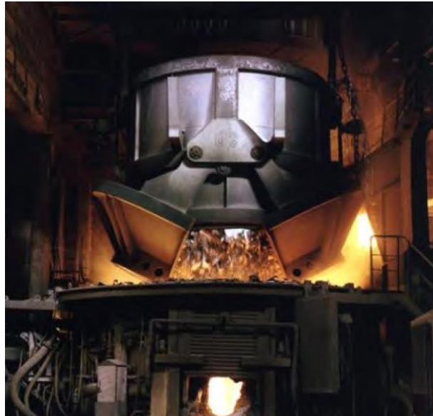
Figura 2 - Cesto a descarregar sucata no forno (Rainer, Miguel et al. 2012).
