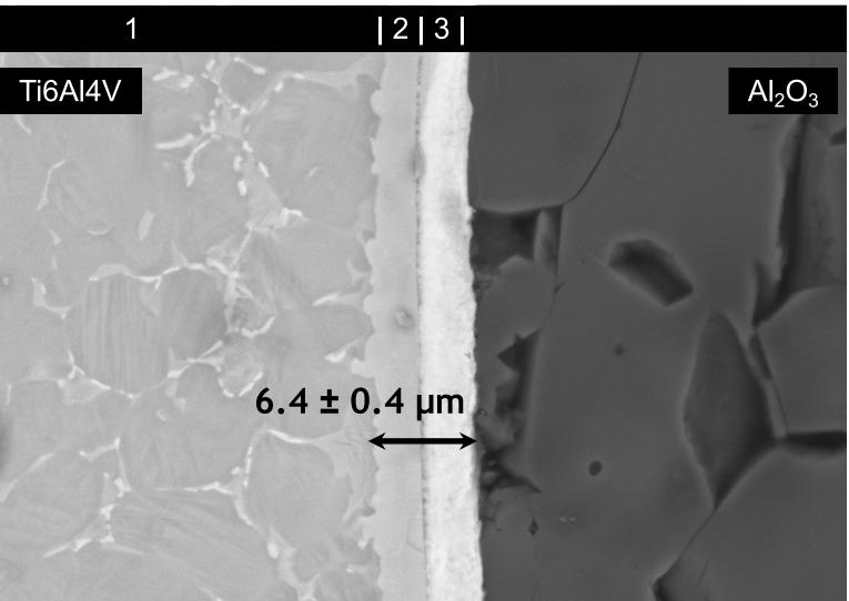
Joined Ti6Al4V to  $Al_2O_3$  using Ni/Ti multilayers with ± 50 nm period with temperature 800°C, pressure of 5 MPa and dwell time 60 min.
