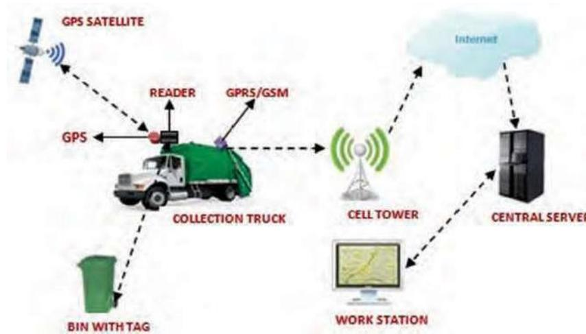
Figure 3: RFID system in MSW management and monitoring;
