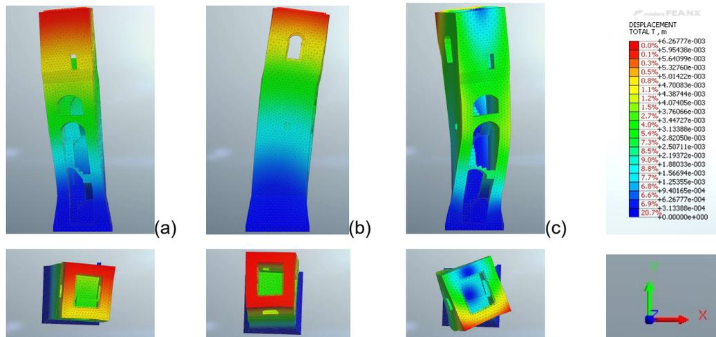
Figure 8 Modal shapes for Model 5. Mode B1,  $f_1=3.95$  Hz (a); Mode B2,  $f_2=4.38$  Hz (b); Mode T1,  $f_3=9.78$  Hz (c). (Figure 9).
