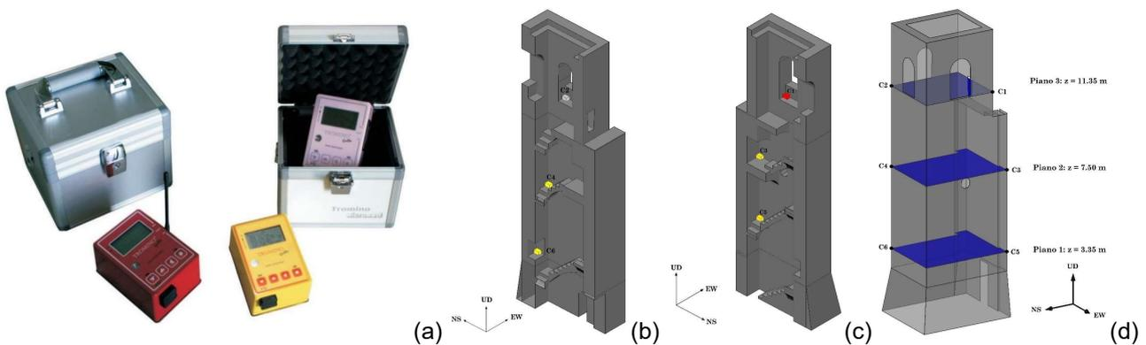
Figure 6. The three types of Tromino used for measurement of the velocity of ambient vibrations (a). The location along two vertical alignments on the opposite corners of the shaft of the tower (b), (c). The identified instrumented levels (d).
