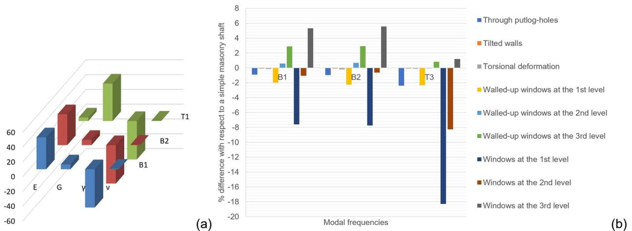
Figure 5. Sensitivity coefficients for orthotropic material mechanical parameters (a) and for architectural details of the model (b) for an ideal tower. B1 is the first bending frequency, B2 is the second bending frequency and T1 is the first torsional frequency.
