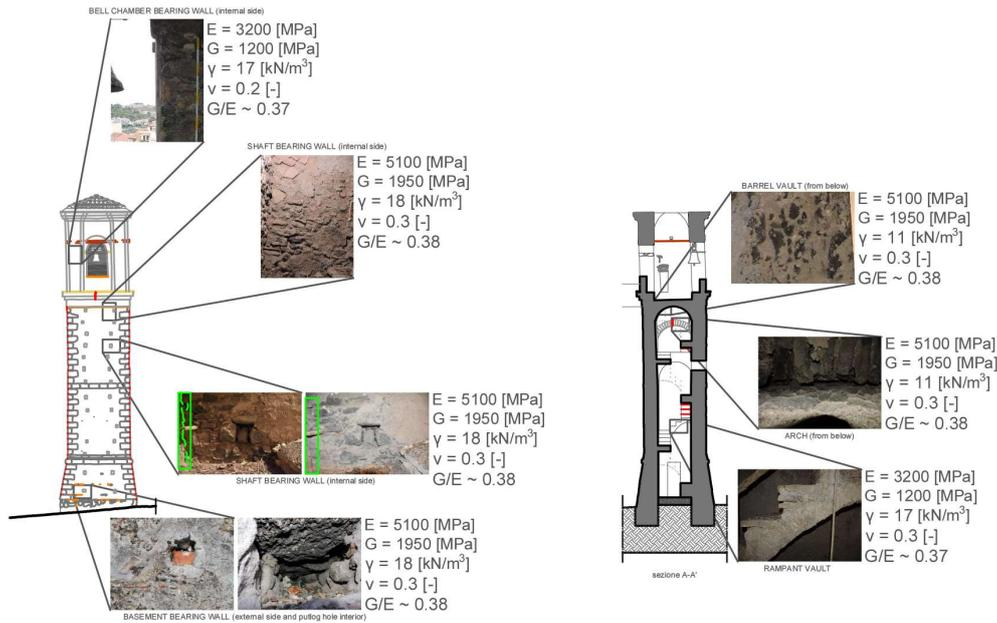
Figure 9. Mechanical parameters attributed to the different parts in the calibrated detailed Model 5, without connection to the church.
