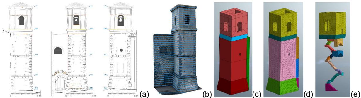
Figure 4. Elevation drawings (a) and 3D textured model from photomodelling with automatically generated horizontal sections (b). High geometric detail 3D model of the tower (c). The 3D model discretized in tetrahedral mesh (d). The mesh of the internal stairs (e).
