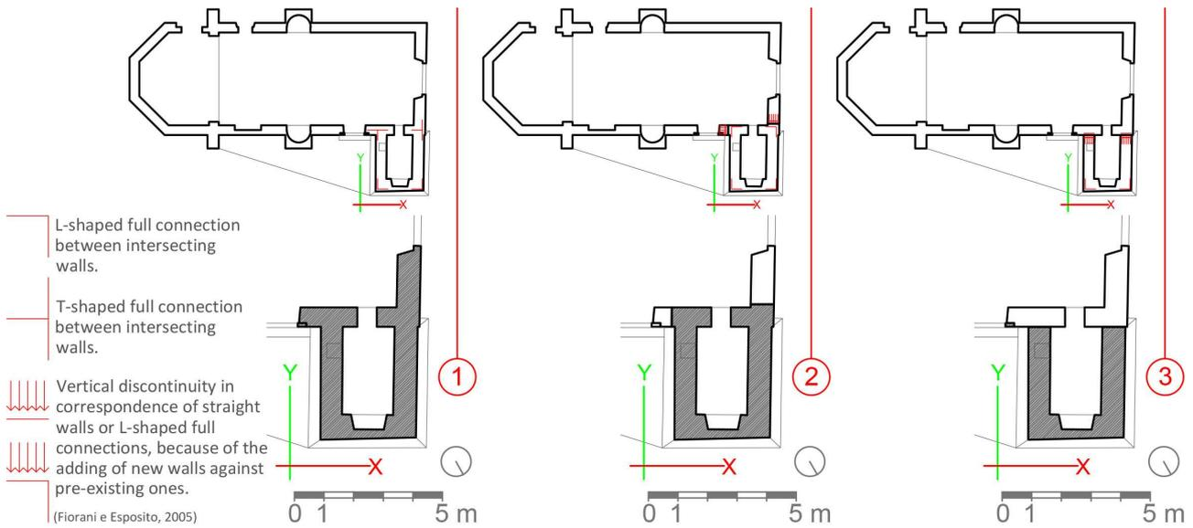
Figure 7. The three different hypotheses about the structural connection between the walls of the tower and the church. (1): Model 1; (2): Model 2; (3): Model 3.
