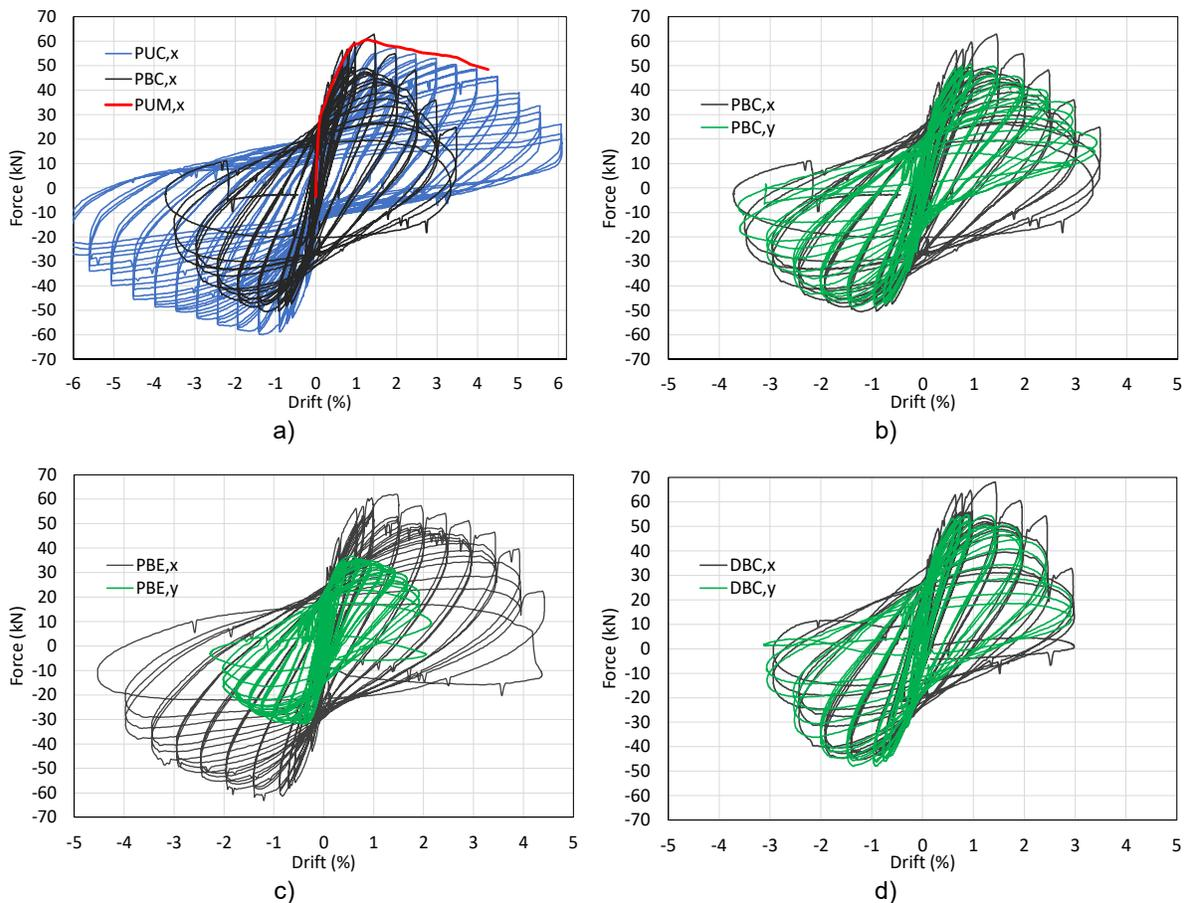
Figure 4. Force – drift relationship: a) uniaxial tests and PBC in x direction; b) column PBC in both directions; c) column PBE in both directions; and d) column DBC in both directions.
