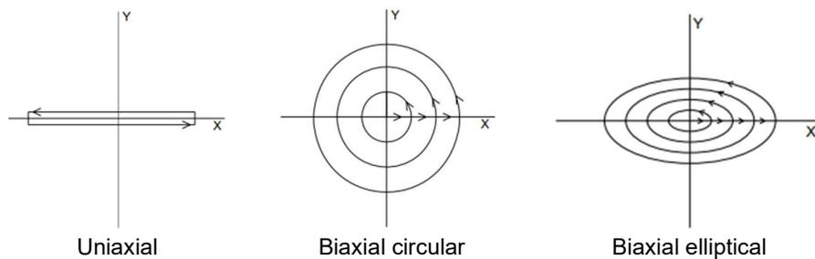
Figure 3. Lateral loading path adopted on the cyclic tests.
