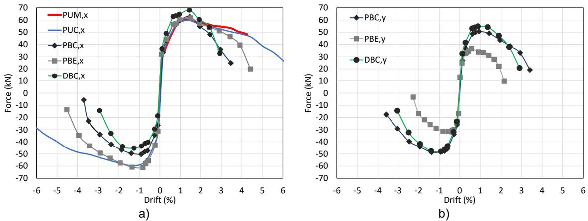
Figure 6. Force – drift envelopes: a) direction x; and b) direction y.
