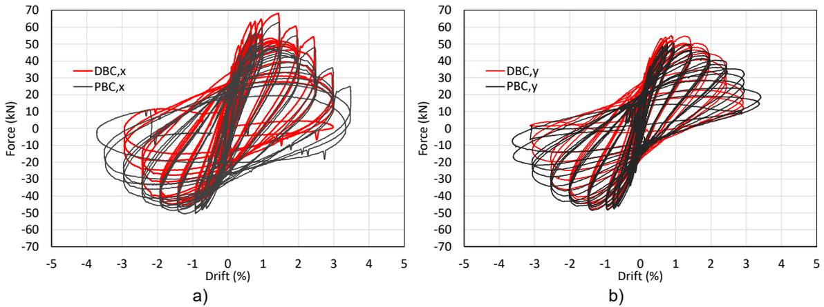
Figure 5. Force – drift relationship for columns PBC and DBC: a) direction x; and b) direction y.
