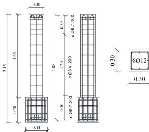
Figure 1. Geometry and reinforcement detailing (dimensions in m).
