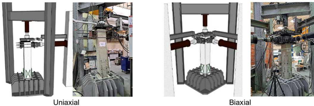
Figure 2. Test setup adopted for uniaxial and biaxial tests.
