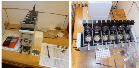
Micro-chamber tests for VOCs emission profile evaluation
