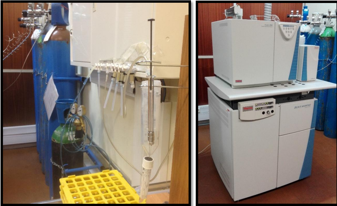
Figure 12. Left - Syringe inserted into the exchanger, pulling 250 \mu\text{L} of air; Right - IRMS system used to measure ^{28}\text{N}_2 , ^{29}\text{N}_2 and ^{30}\text{N}_2 in gas samples;
