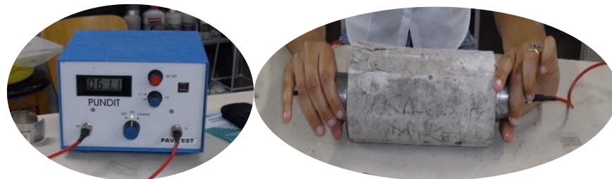
Figure 4. UPV test equipment and stand scheme.
