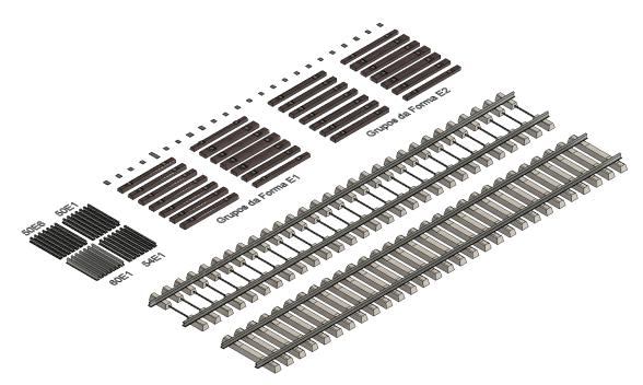
Figure 8 – Railway BIM families for the idBIM4.0 platform
