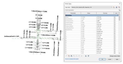
Figure 5 – A geometrically non-parametric 60E1 Vignole rail (according to EN 13674-1:2011+A1:2017)
