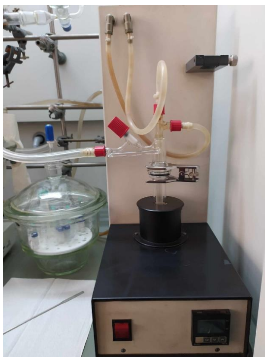
Figure 26. Low pressure sublimator used in this work.
