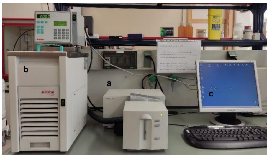
Figure 31. Agilent 8453 UV-Vis Spectrophotometer (a) used in this dissertation. The spectrophotometer is linked to a refrigeration system (b) and to a pc interface (c) for data acquisition.
