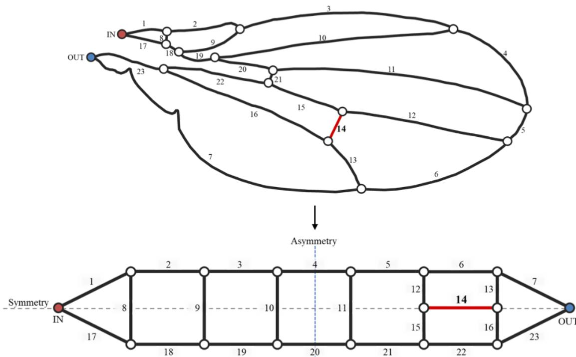
Figure 1 Topological simplification of the wing vein network of a fruit fly, *Drosophila melanogaster*. It is symmetric along an axis shown as the gray dashed line connecting the inlet and outlet but asymmetric along the other axis shown as the blue dashed line which is normal to the former one.
