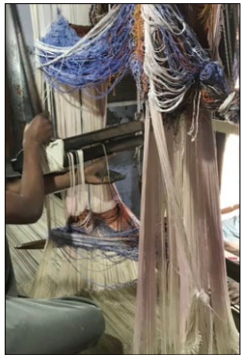
Figure 2b (right) Drawloom with naqsh , Cholapur, Varanasi, India. Photographs: C. Bier, 2020.
