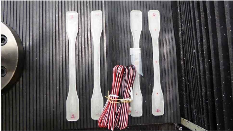
Figure 4.4: Different specimen preparation: specimens 1 and 2 to the left for the clip-on extensometer and 5 and 6 to the right with the strain gauges already mounted on 5.
