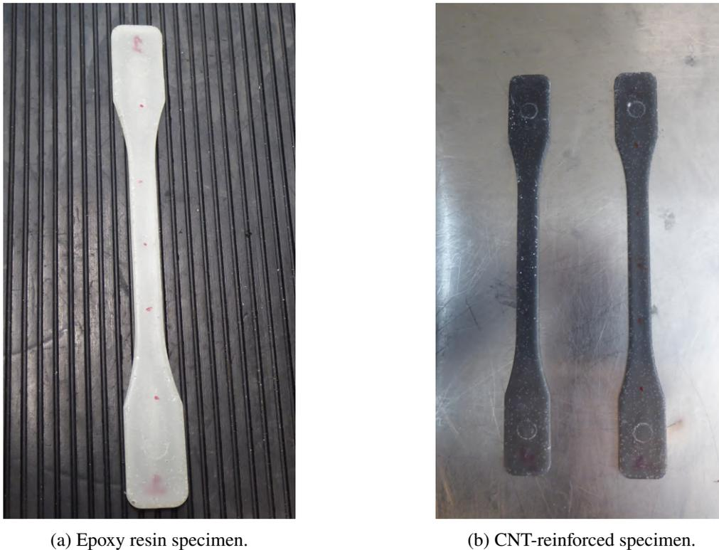
Figure 4.3: Examples of the samples used in the tensile tests.
