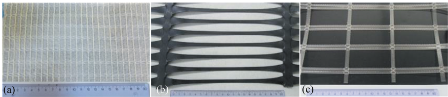
Figure 1. Appearance of the geosynthetics (ruler in centimetres): (a) high-strength composite geotextile (GTX); (b) uniaxial high-density polyethylene geogrid (GG1); (c) polyester geogrid (GG2).
