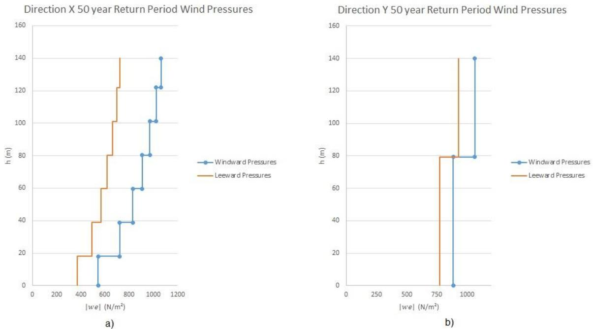
Figure 4.10 – a) Windward and Leeward pressures for the 50 year return period wind action on the X direction, b) Windward and Leeward pressures for the 50 year return period wind action on the Y direction
