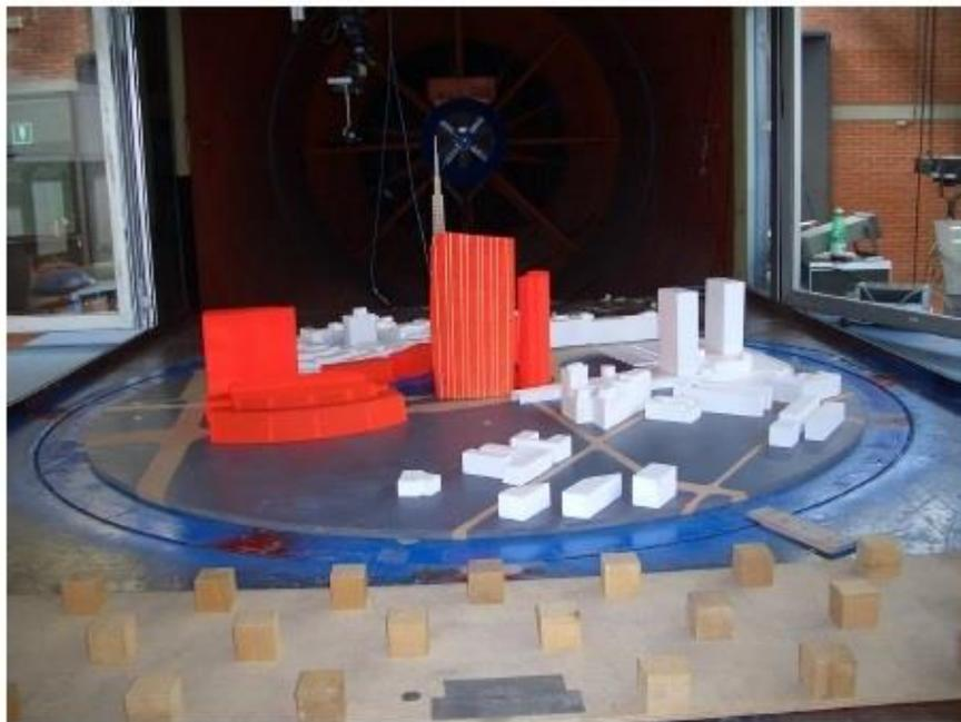
Figure 4.13 – Wind tunnel test 1/350 scaled model [38]
