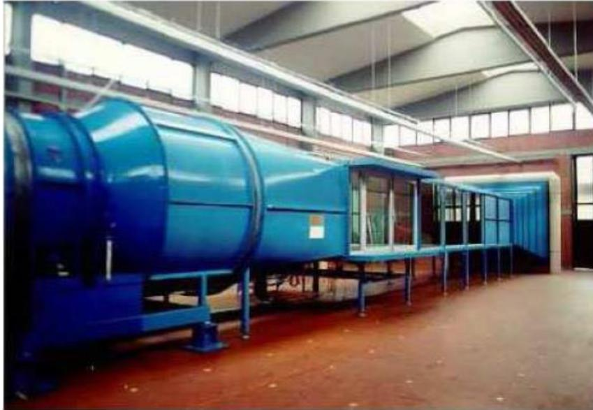
Figure 4.17 – CRIACIV Boundary Layer Wind Tunnel [33]
