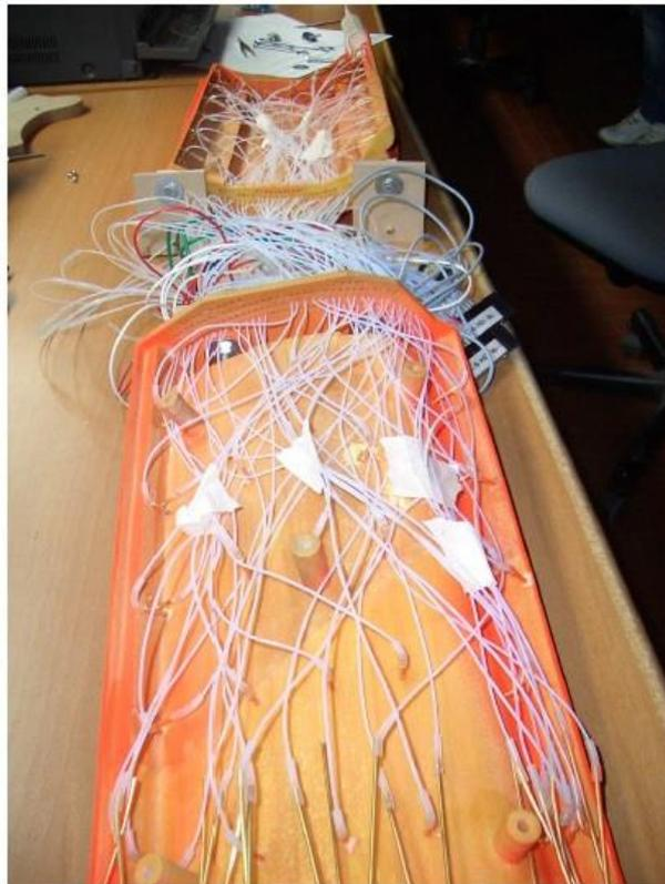
Figure 4.16 – Pressure measurement system [38]
