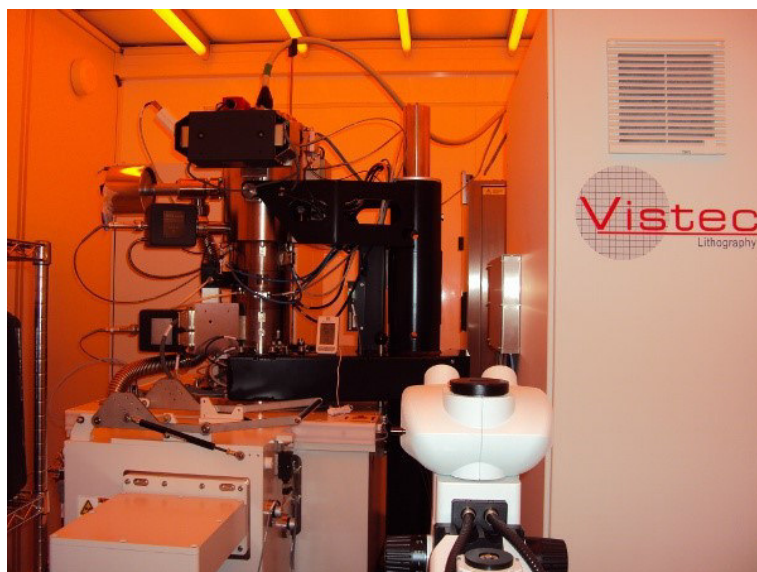
Figure 2.14: e-beam lithography system placed in the INL cleanroom.
