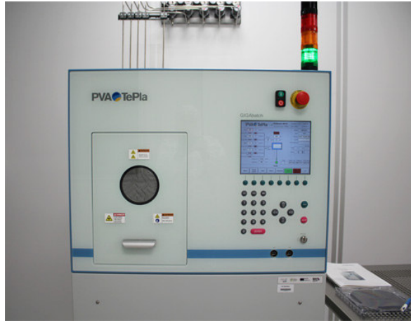
Figure 2.15: Plasma asher system for resist removal located in the INL cleanroom.
