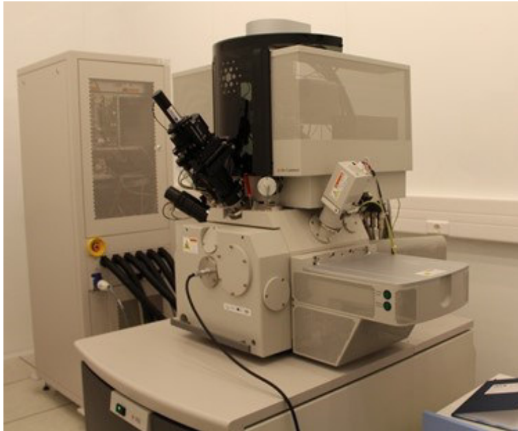
Figure 2.20: FIB with incorporated SEM located in the INL high accuracy laboratories.
