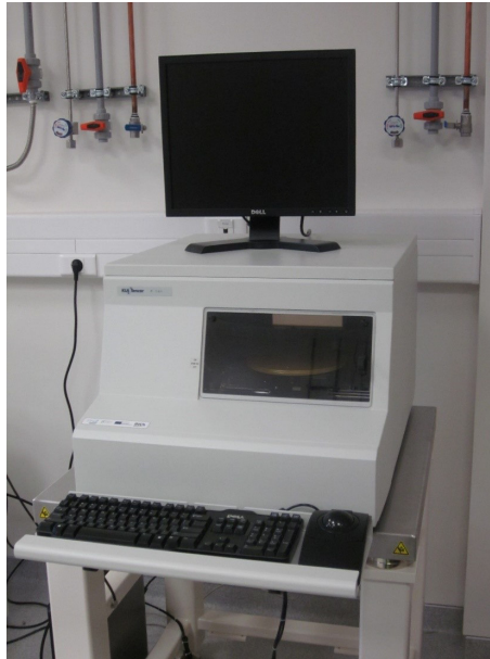
Figure 2.23: Contact profilometer for surface topography characterization (INL cleanroom).
