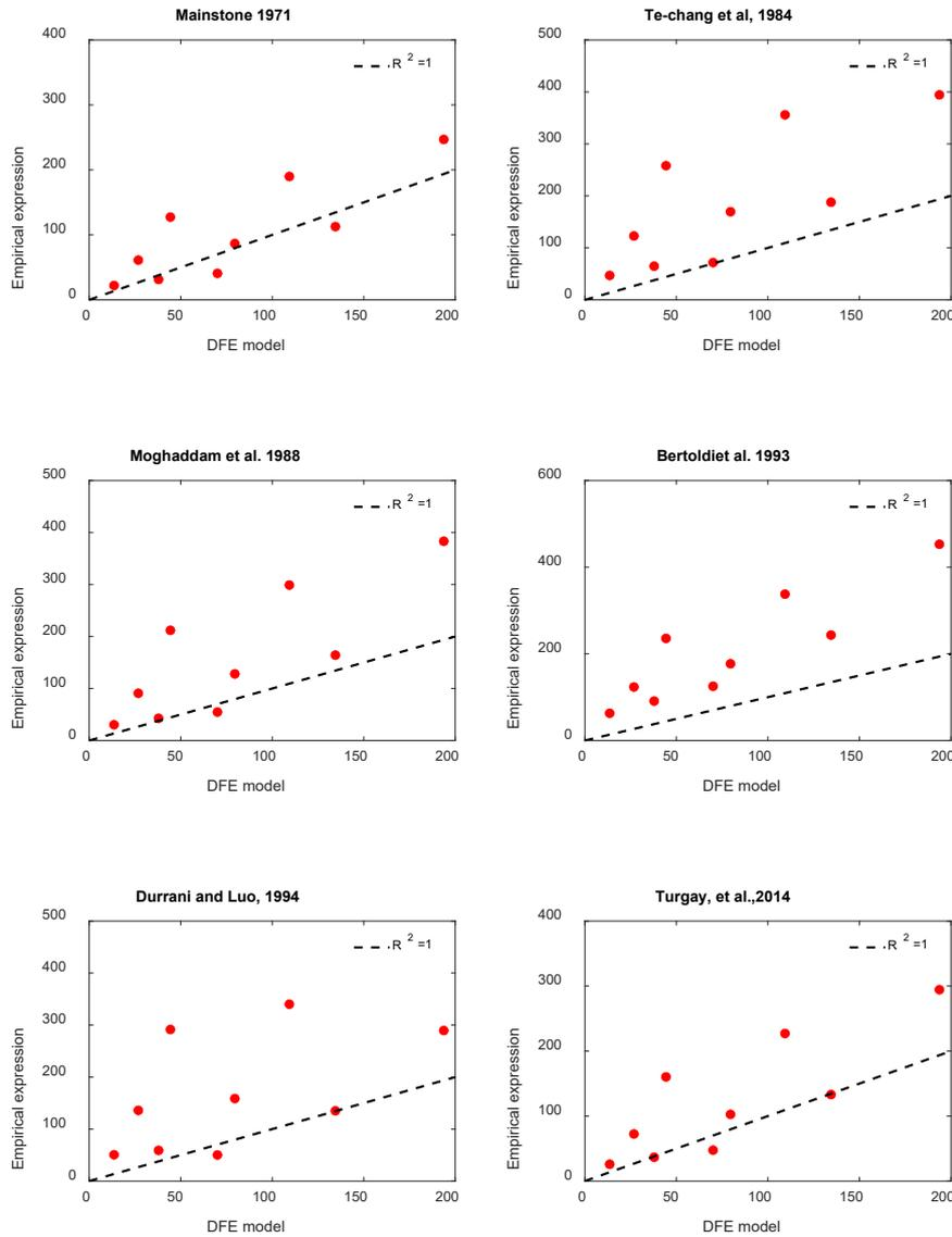
Figure 7 Scatter plots representing estimated infill contribution in terms of strength using different empirical expressions versus the strength obtained from the detailed finite element model.
