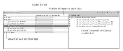
Figure 1 – Eclipse Plug-in RZoltar View
