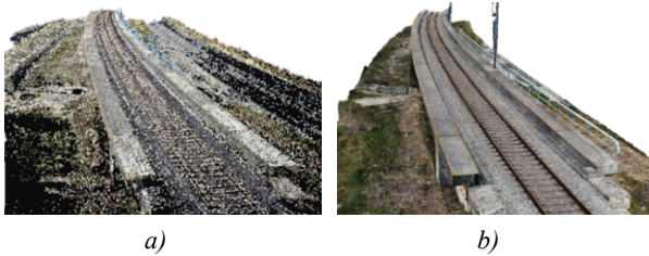
Figure 8: Outputs: a) dense point cloud b) texture map
