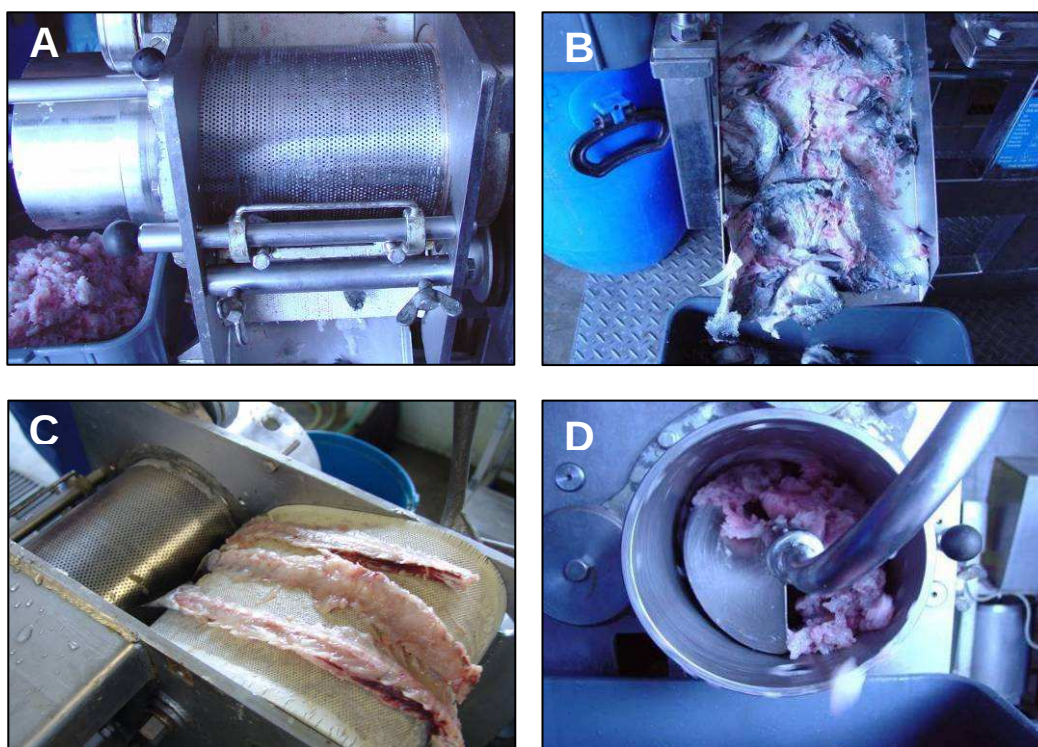
Figure 1.6 – Baader flesh-bone separator. A – General view; B – Discarded material; C – Feeding area; and D – Perforated drum and mince production (pictures from: IPIMAR).
