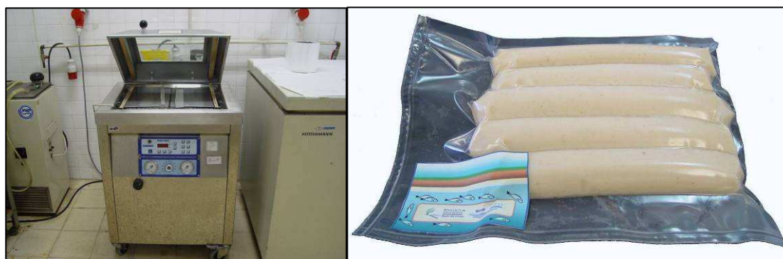
Figure 6.16 – Vacuum-pack device and vacuum-packed product (pictures from: IPIMAR).
