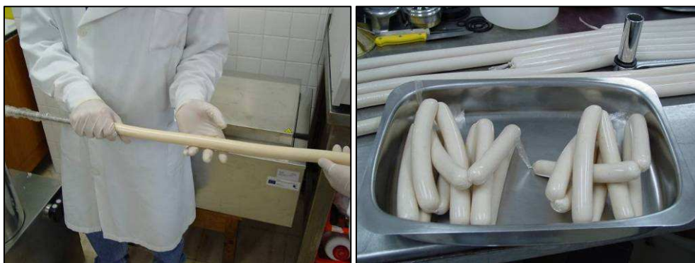
Figure 1.16 – Encasing, twisting and tying of fish Frankfurter sausages (pictures from: IPIMAR).
