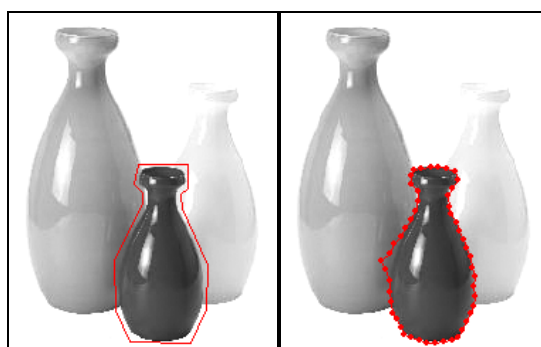
Fig. 5: Initial contour (left); result of the segmentation with k=2,000\text{N/m} considering a model with 50 nodes and made of rubber (right).
